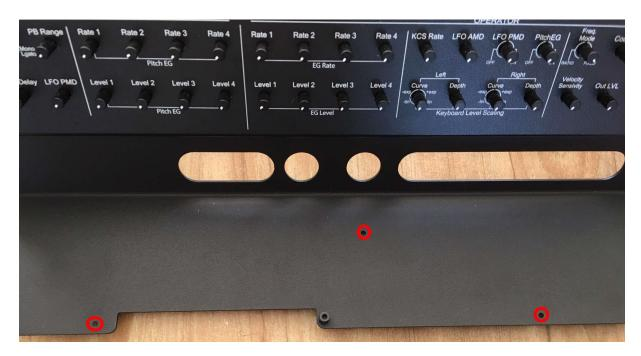
1) Remove these 3 screws and posts from the RDX programmer
