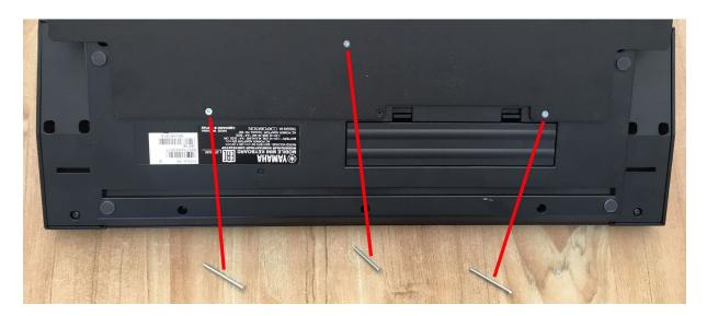
3) Mount the RDX as shown, using the 2 long (M3x40) screws on the outside and the 1 short (M3x30) in the middle.
