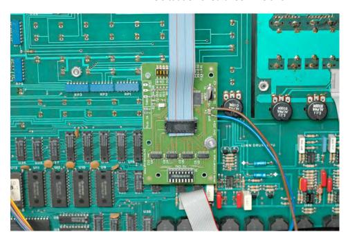
• Connect the blue and brown wire to the capacitor for the power.
